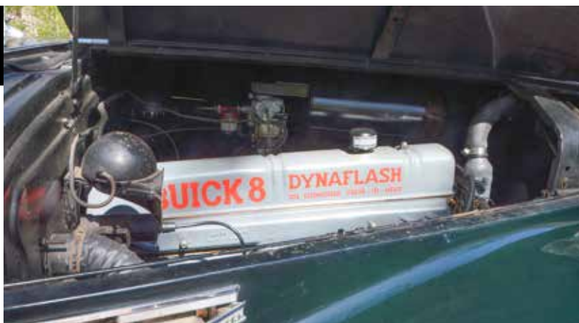
The Roadmaster's Dynaflash engine—a straight-eight marvel—was renowned for its smoothness and power capable of propelling this automobile to impressive speeds for its time, with a top speed that flirted with 100 mph
