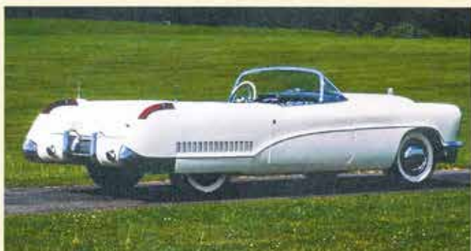
1953 Buick Wildcat - Designed for the 1953 Motorama, the Wildcat is a low-slung, two-seat convertible with a raked wraparound windshield and a hydraulically operated top.
