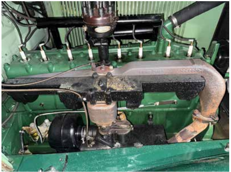
The eight-cylinder engine runs strong, smooth, and quiet on nine main bearings, producing 122 horsepower at 3,200 rpm, and is mounted on a double-drop chassis with automatic clutch and Houdaille shock absorbers.
