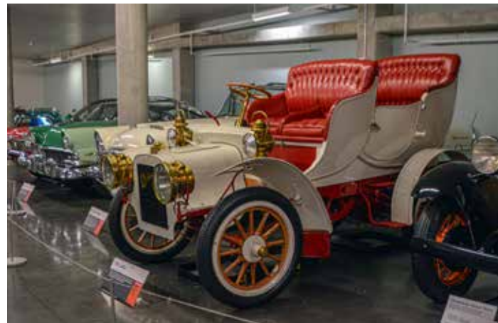
1906 Cadillac Model M, Tulip Tourer, 5-Passenger 1 cylinder, 98.2 cu in, 10 hp, 2 speed planetary
