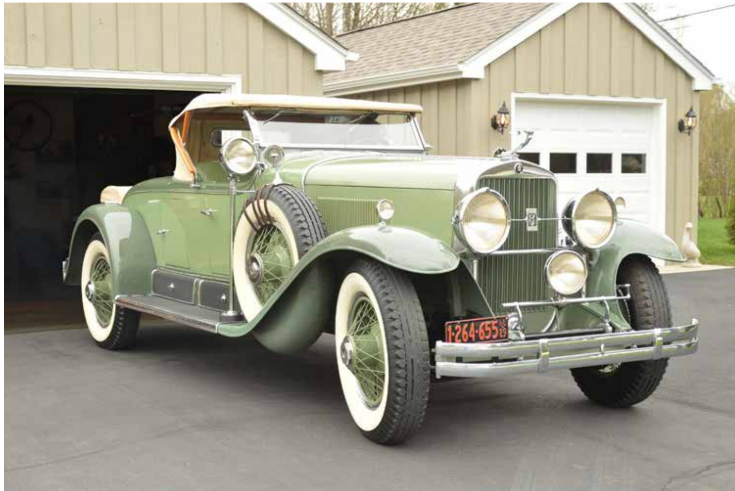
1929 Cadillac Sport Roadster Model "341B" 90 Horsepower, V8 140 Inch Wheelbase, Weight 4,678 Lbs Cost New $3,350
