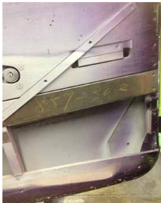
A wiring diagram and an assortment of parts. Below is the inside of the door, with the original chalk markings 859-302, which match the car's data plate.
