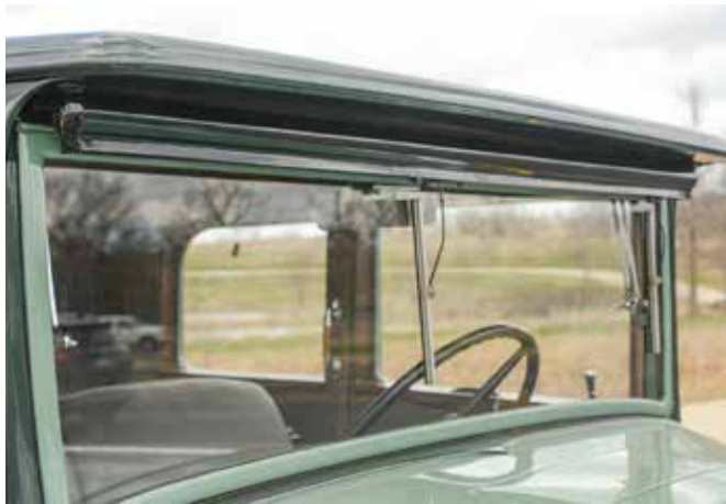
A Trico Visionall Wiper system features three wiper blades that use engine vacuum to move the wipers side to side.
