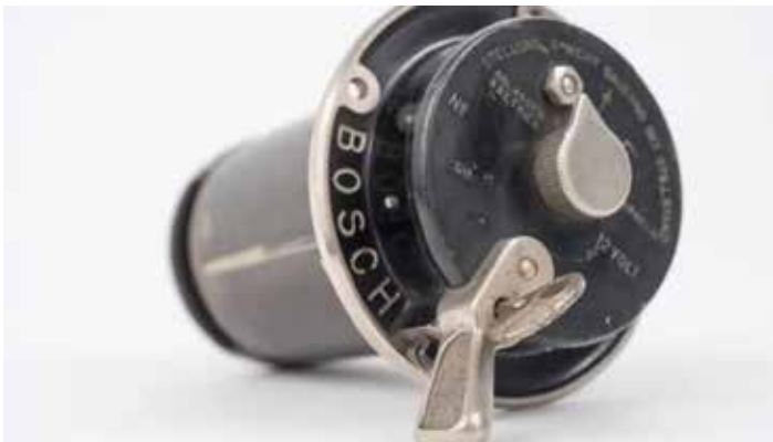
1911 - lockable ignition coil
