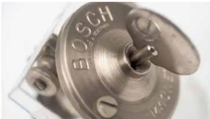
1912 separate ignition lock, fitted discreetly to dashboard
