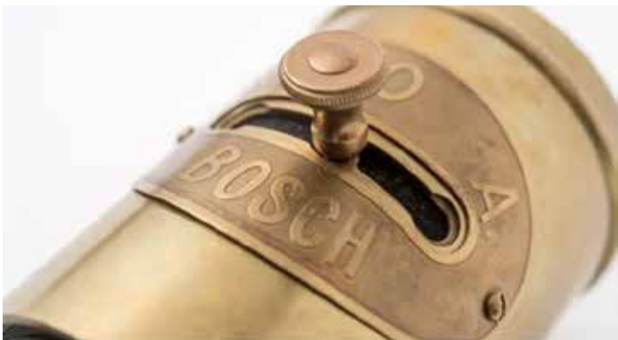
Bosch ignition coil for automobile ignition systems 1908
