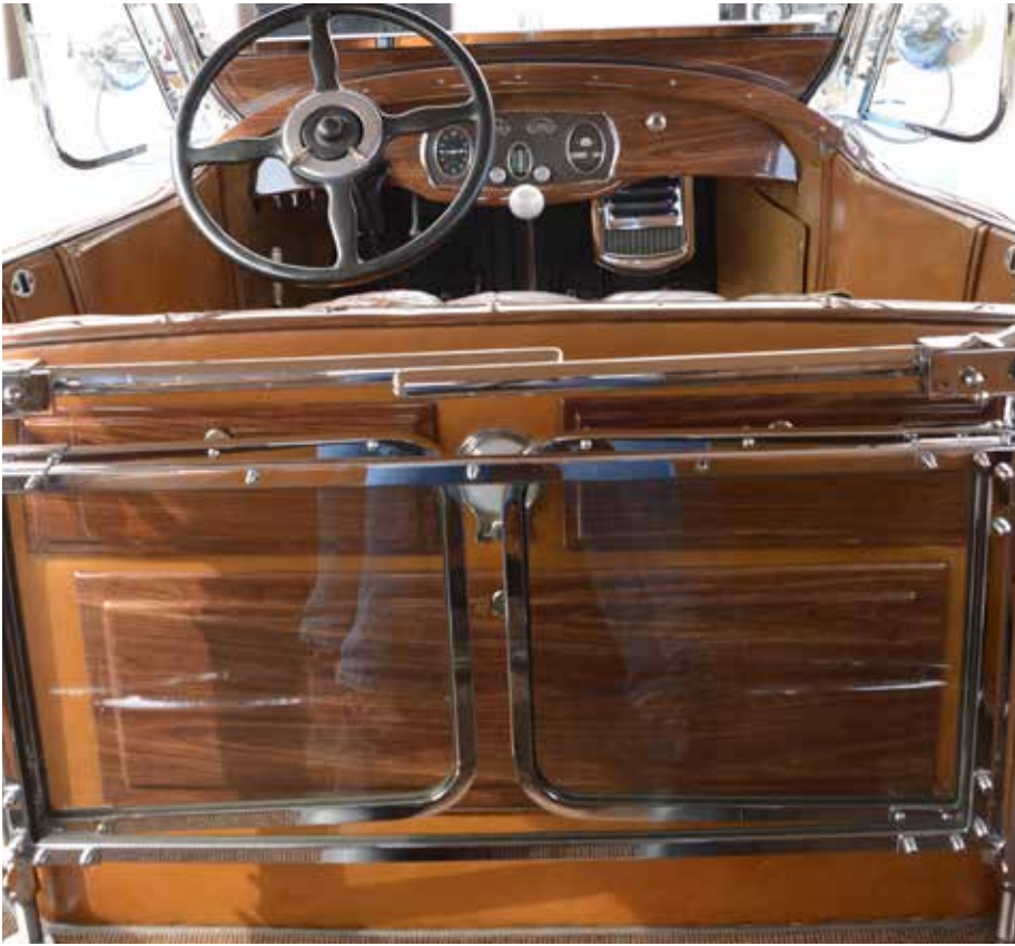
The interior tonneau windshield, shown in the down position.
