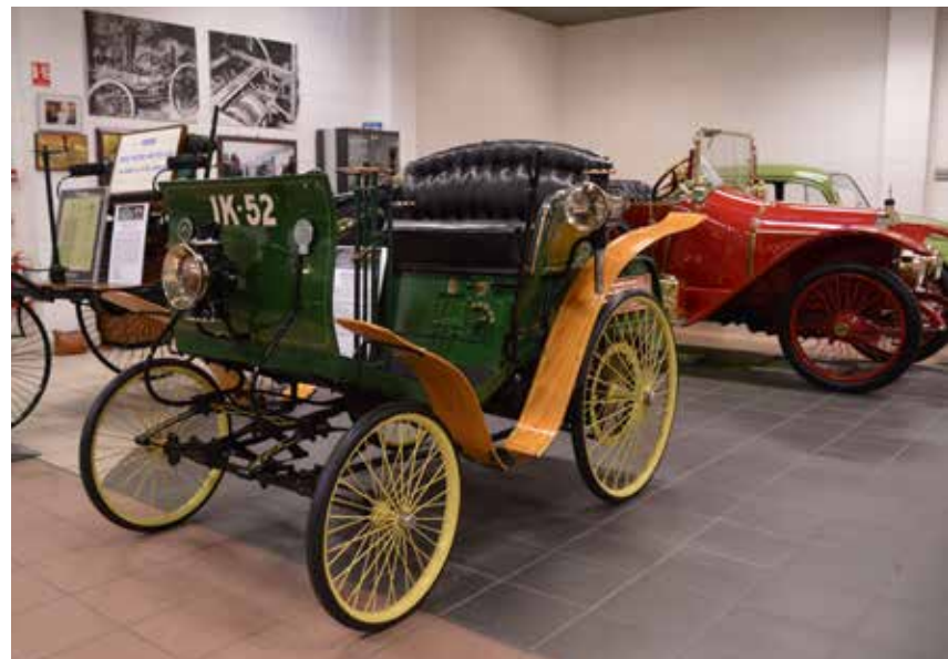
1 cyl engine; weight: 617 lbs; top speed: 16 mph Production: 1200 (1894 - 1899)
