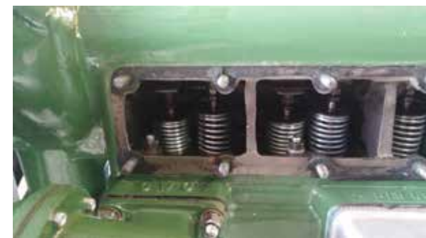
Upper engine front cross section with single intake valve
