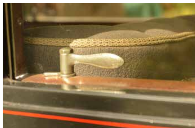
The door handles on the window frame pivot, allowing the door to be opened.
